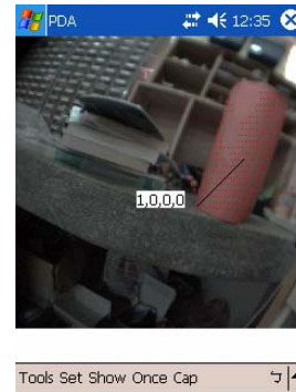
Figure 9: Picture of recognizing the red color.
