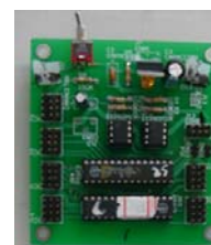
Figure 7: Photo of gait synchronization controller.
