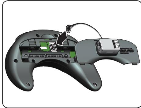
An image of the BT-410 installed in the RC-100B
