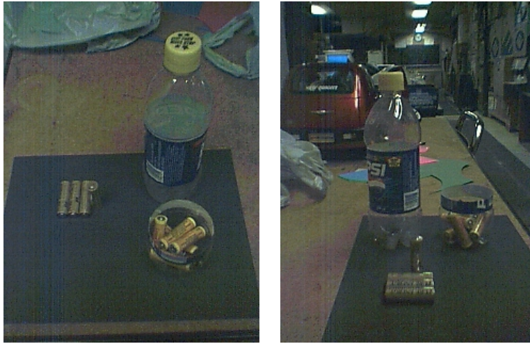
Figure 3: A suitable basket for the lift and carry challenge on the right and suitable weights (Standard AA batteries) in front. Such a basket must be fitted to the robot before the lift and carry challenge. A standard 591ml soft drink bottle is shown for comparison. The basket in the picture was constructed by cutting the bottom off the soft drink bottle.
